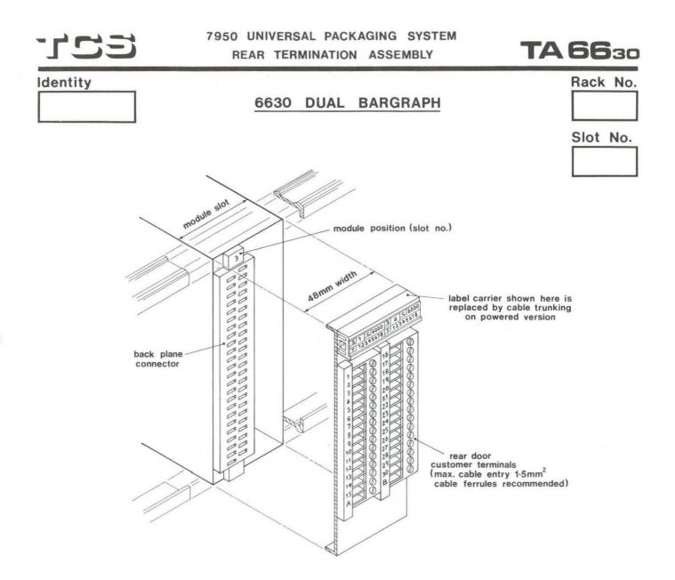
The TA6630 termination assembly consists of a 48 pin back-plane connector with a wire loom linking the module connections on the back-plane to three rows of 16 customer terminals. The assembly is used to mount 6630 Dual Bargraph Indicators into the 7950 Universal Packaging System.
