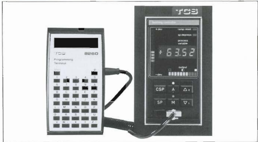
The photograph shows an 8260 terminal plugged into the front panel of a 6352 controller. A full list of the available command parameters is given in the 6352 Facts Card.
