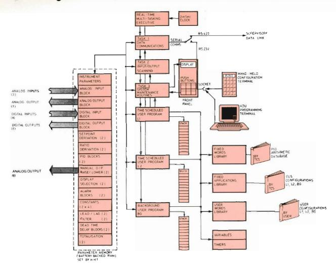
The 6366 supports two time scheduled programs and a background program. These are selected using the hand-held terminal by setting their names into the parameters L1, L2 and BG in the general purpose parameters block.
