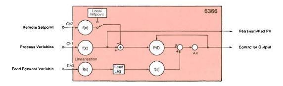
The example shows a single PID control loop with both internal and remote setpoints. The third channel is used for a feed forward variable that modifies the control output.
