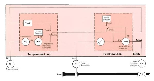
The example shows a process temperature being controlled through a secondary fuel flow loop using one 6366 controller
