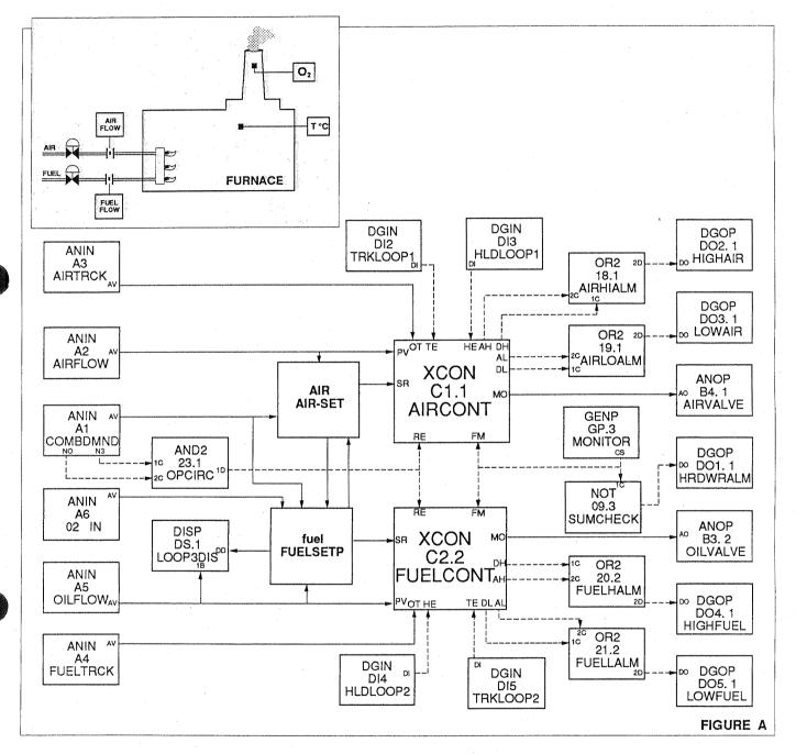
**FIGURE A** The scheme illustrated is single fuel with fuel/air cross-limiting and oxygen trim.
