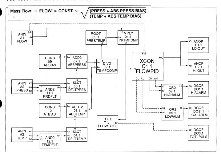
The pressure and temperature compensation signals are fed in and referred to absolute terms. The resultant compensation is applied to the raw flow signal which is then used as the control function PV. If either the temperature or pressure signals go 'open circuit' default signals are automatically selected. If the flow signal goes 'open circuit' the controller enters 'forced manual' mode to give fail-safe operation.
