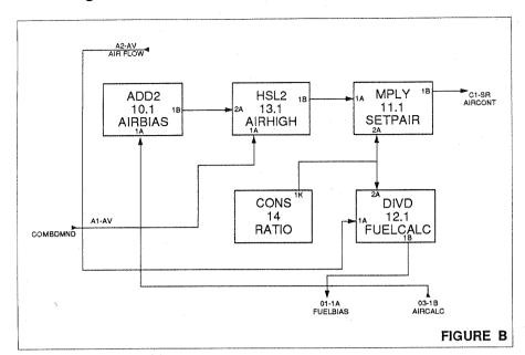
FIGURE B The air relational control is run in a compound called AIR-SET in which the lead-lag, air bias, and air ratio functions are handled with respect to the combustion demand signal and the fuel rate. AIR-SET also calculates the fuel bias signal used to modify the fuel rate.
