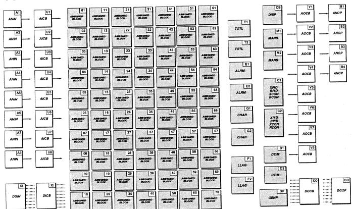
The larger set of fixed blocks in the 6372 and 6382 series of instruments includes Analogue Input (ANIN) and Analogue Output (ANOP) blocks, an 8-way Digital Input (DGIN) block, an 8-way Digital Output (DGOP) block, Control (XPID, RPID, XCON, or RCON) blocks, Manual Station (MANS) blocks,
