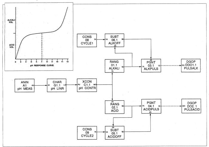
The pH measurement is fed into a 16-breakpoint Characterisation (CHAR) block to condition the signal. This signal is then fed into the PV of the control block with the manual station output (MO) going to the acid and alkali range (RANG) blocks. These determine the requirement to dose either
