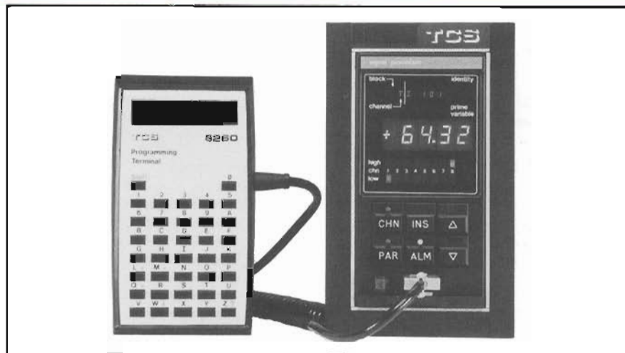
The photograph shows an 8260 terminal plugged into the front panel of a 6432 processor. A full list of the available command parameters is given in the 6432 Facts Card.
