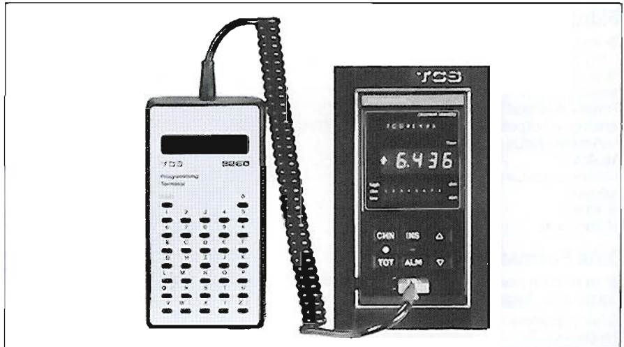
The photograph shows an 8260 terminal plugged into the front panel of a 6436. A full list of the available command parameters is given in the 6436/7 Facts Card.
